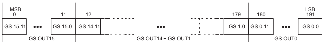
Figure 17. Grayscale Data Packet Format
